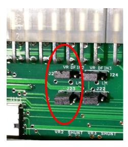
And this is the same thing for the expansion connector pin #24 with the "Digital Frequency Input 3. The expansion connector pin #23 named "VR DFIN3 —" is normally connected to the second wire of the VR sensor.
